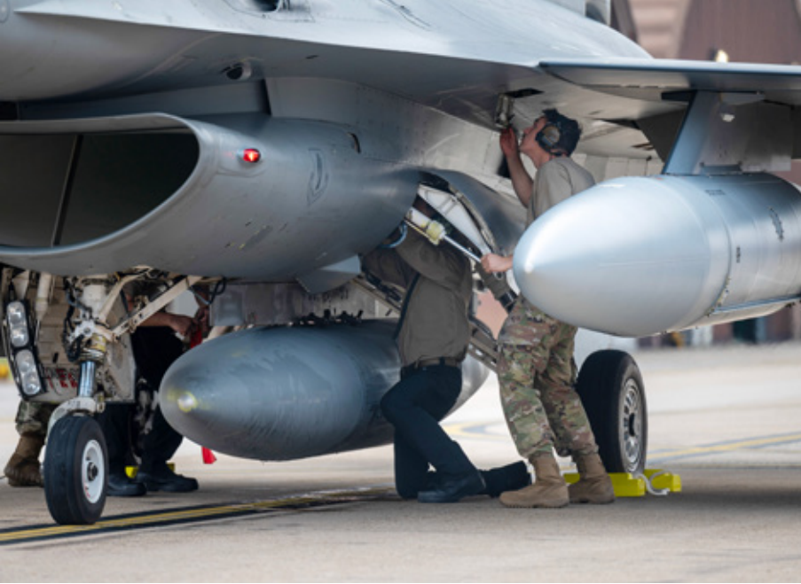
U.S. Air Force Senior Airman Rowley Corbin, 25th Fighter Generation Squadron F-16 Fighting Falcon assistant dedicated chief, inspects an F-16 assigned to the 13th Fighter Squadron at Osan Air Base, Republic of Korea, June 26, 2025. The F-16s were transferred from Misawa Air Base, Japan and have undergone a series of avionics system upgrades, bringing the aircraft closer to fifth-generation capabilities as they increase both the survivability and accuracy of the weapon system. ▲
